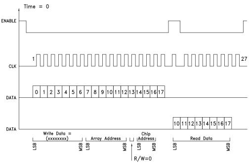
Figure 23. Timing Diagram for reading a row of the Transmitter Serial Interface
