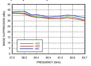
Figure 16. Carrier Suppression vs. Frequency Over Temperature<sup>[6][8]</sup>
