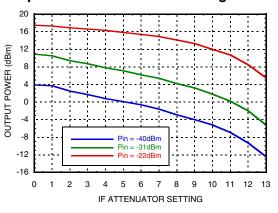
Figure 10. 62.64 GHz (IEEE CH-3) Output Power vs. IF Gain Setting<sup>[3][4]</sup>
