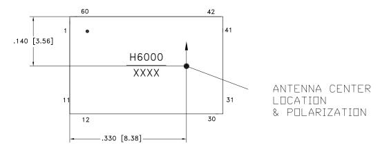
The antenna is located inside the package with geometric center and linear polarization angle as shown. The geometric center can be used as the antenna pattern phase center provided there is sufficient unobstructed ground plane extension around the chip. Measured antenna pattern phase centers will vary with frequecy and are dependent on finite ground plane effects, and coupling to nearby components.
