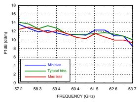
Figure 9. 60.48 GHz (IEEE CH-2) Output Power vs. IF Gain Setting<sup>[3][4]</sup>
