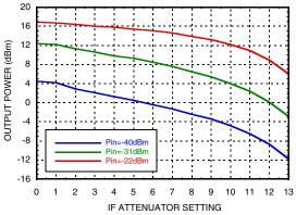
[3] Input power of -40, -31, and -22dBm applied at each of the 4 baseband inputs.[4] Measured without antenna gain.
