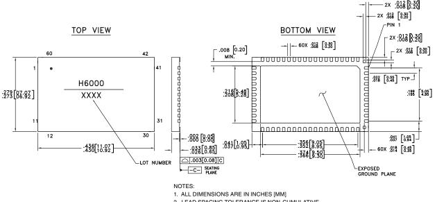
2. LEAD SPACING TOLERANCE IS NON-CUMULATIVE.
