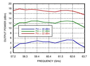
Figure 7. P1dB vs. Frequency Across Voltage<sup>[4]</sup>
