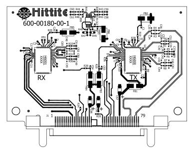
The circuit board used in the application should use RF circuit design techniques. Signal lines should have 50 Ohm impedance while the package ground leads and exposed paddle should be connected directly to the ground plane similar to that shown. A sufficient number of via holes should be used to connect the top and bottom ground planes. The evaluation circuit board shown is part of an evaluation kit available from Hittite.
